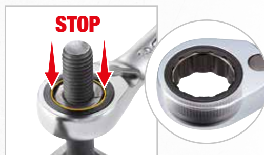
SPRING STEEL RING INTEGRATED in the bihexagonal head for better grip
