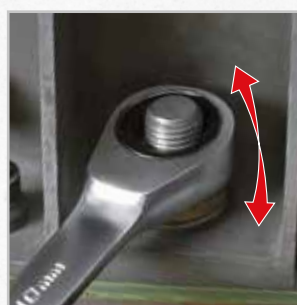
CHANGE OF ROTATION DIRECTION reversing the key 180°
